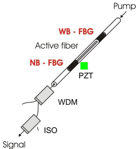
Figure 3.2 Laser Schematic
