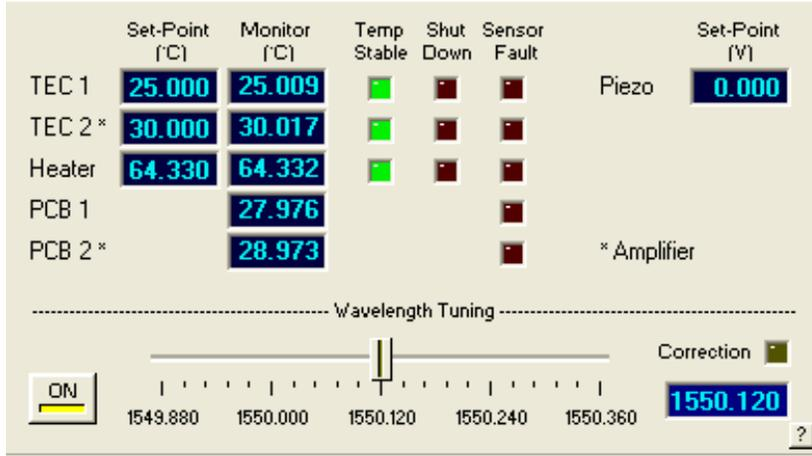
The Temperature Control section comprises a series of numerical readouts and status indicators associated with the Seed laser’s temperature control and monitoring functions.
