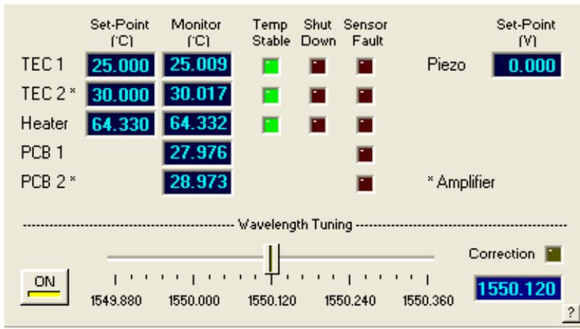
When Wavelength Tuning is switched ON the slider can be used to control the Seed laser wavelength. When the slider is moved the Seed Heater temperature and Piezo voltage are tuned according to an internal calibration to avoid second mode regions and reach the calibrated wavelength.
