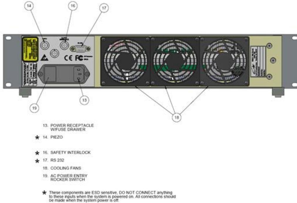
Figure 5.2 Rear Panel of the Fiber Laser Source
