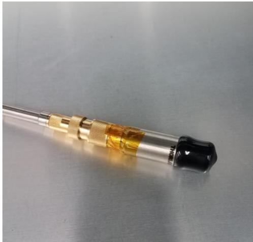
**For RFLPXA systems with less than 1W output power output (or multi fiber output with less than 1W per fiber), the fiber can either be coupled to a free-space collimator or connected to another fiber patchcord. Make sure that the laser is turned off before making any connections.**
