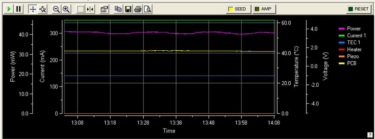
Figure 7.4 Display Window – Seed Laser Parameters
