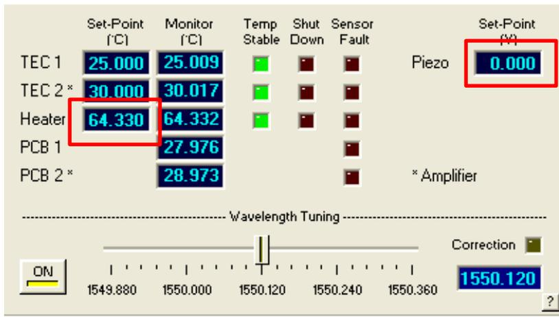
With the wavelength tuning turned off, it is possible to type in values in the *Heater* set point box and the *Piezo Drive* set point box and press the return key. The numerical wavelength display is invalid.
